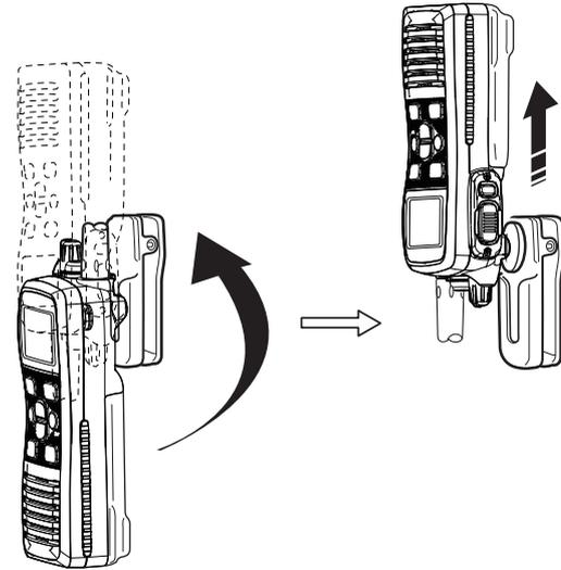
**⚠ CAUTION: HOLD THE TRANSCEIVER TIGHTLY WHEN HANGING OR DETACHING THE TRANSCEIVER FROM THE BELT CLIP.**
