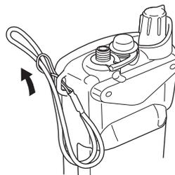
Pass the handstrap through the loop on the top corner of the transceiver, as illustrated to the left. This facilitates carrying the transceiver.
