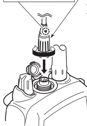
**CAUTION:** Attach the speaker-microphone's connector securely to prevent accidental dropping, or water intrusion in the connector.
