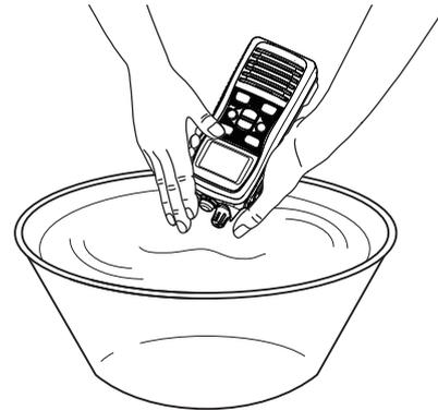
**NOTE: DO NOT** wash the transceiver in water if there is any reason to suspect the waterproofing may not be effective. For example, in cases where the [SP MIC] jack cover is damaged, the transceiver/battery pack is cracked or broken, or has been dropped, or when the battery pack is detached from the transceiver.
