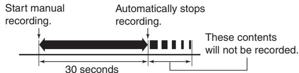
30 seconds after you start the manual recording, the recording will automatically stop.
