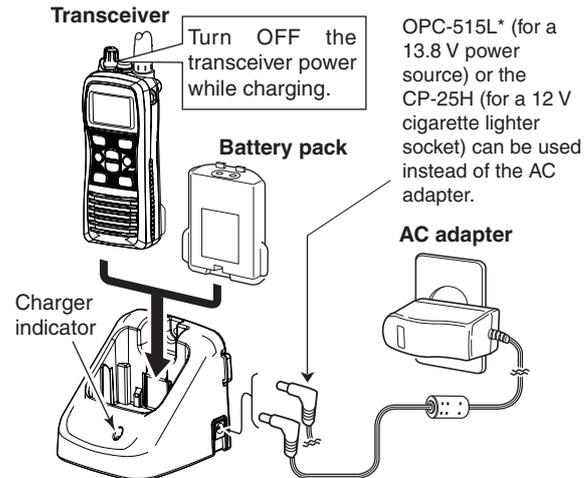
\* **CAUTION: NEVER** connect the OPC-515L to a power source using reverse polarity. This will ruin the battery charger.
